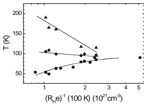
Figure 2. Temperature versus doping phase diagram obtained from transport measurements.  $T_c$  (circles), the pseudogap temperature  $T^*$  (triangles) and  $T'$  (diamonds).
