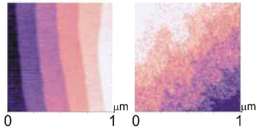
Figure 1. AFM topographic images of, (left), an etched  $\text{SrTiO}_3$  substrate showing atomically smooth terraces and, (right), a 5 nm thick  $\text{Pb}(\text{Zr}_{0.2}\text{Ti}_{0.8})\text{O}_3$  film, grown onto an etched substrate and a thin metallic  $\text{SrRuO}_3$  buffer layer. The height between each terrace is 0.4 nm, corresponding to one unit-cell.
