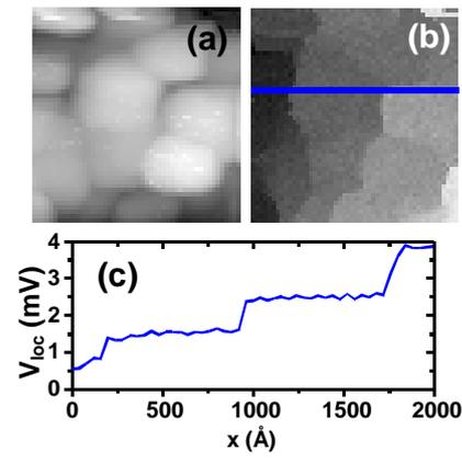
Fig.2. Topographic (a) and potentiometric (b)  $2000 \times 2000 \text{ \AA}$  images of a LSMO/MgO textured thin film acquired with an applied electric field of 17.6V/mm. gray scale: a) 18nm, b) 4mV. (c) Potential profile along the path in b).
