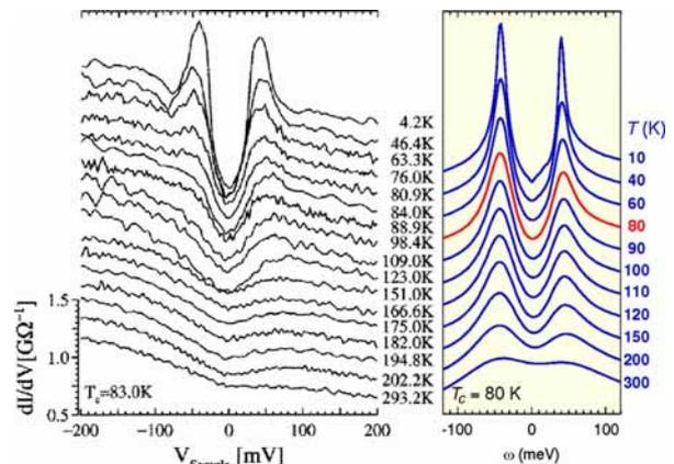
Tunneling spectra across  $T_c$ . Left: experimental data from Renner *et al.*, Phys. Rev. Lett. **80**, 149 (1998). Right: theoretical result based on the Cooperon propagator description of d-wave superconductivity.
