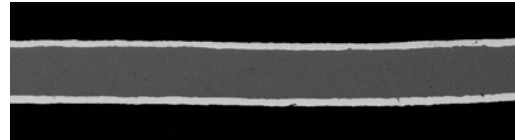
Figure 5: {110}<011> textured Ag/NiCrV/Ag ribbon. The total thickness is 60µm.
