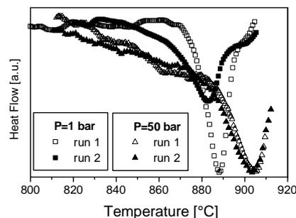
Figure 2: DTA traces of two subsequent temperature ramps melting a  $\text{Bi,Pb(2223)}$  sample. A pressurised atmosphere renders the process reversible.
