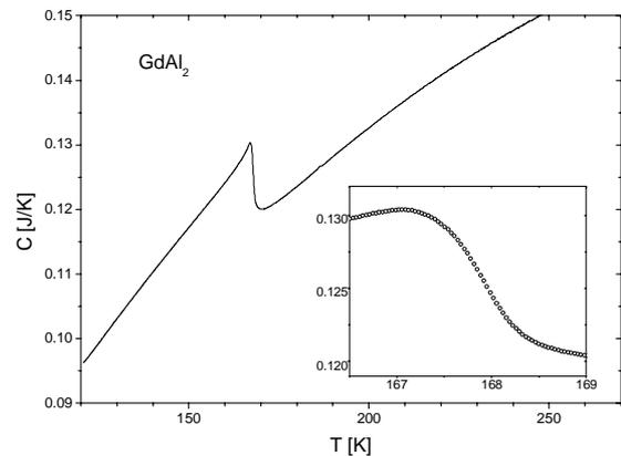
Fig. 5: Heat capacity of a  $\text{GdAl}_2$ .
