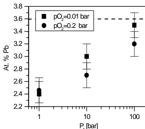
Figure 3: Pb-content of  $\text{Bi,Pb(2223)}$  after heating above the decomposition temperature, plotted against the gas pressure in which the samples were treated.
