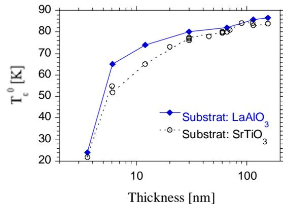
Fig.1:  $T_c$  dependence in function of the thickness of the  $\text{NdBa}_2\text{Cu}_3\text{O}_7$  thin films for two substrates
