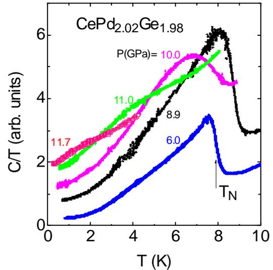
Figure 3. The inverse lock-in voltage  $V_{ac}^{-1} \propto C/T$  of  $\text{CePd}_{2.02}\text{Ge}_{1.98}$  at selected pressures. The Néel temperature,  $T_N$  (5.1 K at  $P = 0$ ), reaches its maximum at 9 GPa. At higher pressure  $T_N$  decreases. On approaching the magnetic quantum critical point at  $P_c \approx 12$  GPa, signatures of magnetic ordering broaden. Above  $P_c$ ,  $C/T$  becomes flat and decreases by a factor of about 5.
