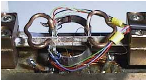
Figure 1: Detail of the head of the sample holder with the extensometer clamped on the sample support
