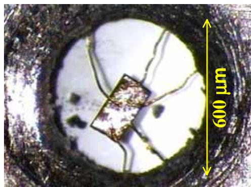
Figure 1. DAC containing a  $200 \times 120 \times 20 \mu\text{m}$   $\text{CeCu}_2\text{Si}_2$  crystal. Five  $10 \mu\text{m}$  gold wires have been spot welded to the sample, enabling two independent 4-point resistance measurements to be taken. The wires are insulated from stainless steel gasket by a layer of alumina powder and epoxy resin. Emission lines from ruby grains placed in the cell provide a direct measurement of the pressure.
