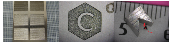
Figure 37: Left: abrasive structures in hard coating (for tools like files). Center: a decorative logo in hard surface alloy (polygon size 6 mm). Right: a small cutting die machined by wire-EDM, a tungsten coating was produced using a tungsten wire electrode.
