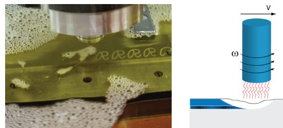
Figure 35: In a first step, bulk, cylindrical electrodes have been used to explore the coating parameters. The use of simple, rod-shaped electrodes avoids the costly and time-consuming process of dedicated wire fabrication in the research phase.
