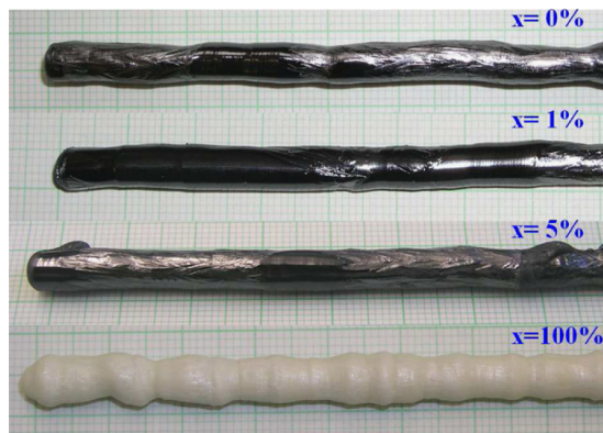
Figure 3: As grown single-crystals of Bi(Cu 1-x Zn x ) 2 PO 6 ( x = 0\% , 1\% , 5\% ), together with a rod of BiZn 2 PO 6 .
