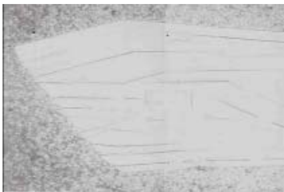
Fig.5. 20 \mu\text{m} thick slab of \text{Bi}_2\text{Sr}_2\text{Ca}_{0.92}\text{Y}_{0.08}\text{Cu}_2\text{O}_8 which was cut perpendicular to the planes. The gray area surrounding the slab is stycast, which serves to support this brittle material. The sample with stycast was mounted on a conical sample holder of the kind shown in Fig. 4.
