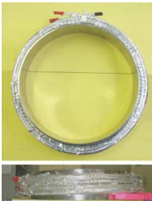
Fig. E-1. Double pancake coils made of Bi,Pb(2223)/Ag. (R. Flükiger, UniGE, project 3).
