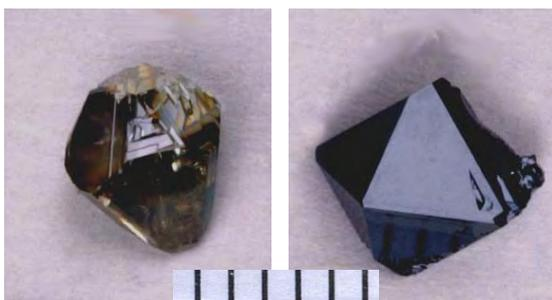
**Figure 16:** Large single crystals of anatase (left) and rutile (right) phases of TiO<sub>2</sub>.
