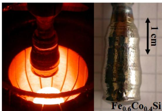
**Figure 8:** Crystal growth of  $(\text{Fe,Co})\text{Si}$  from levitating melt (left). As-grown crystal boule of  $\text{Fe}_{0.6}\text{Co}_{0.4}\text{Si}$  (right).
