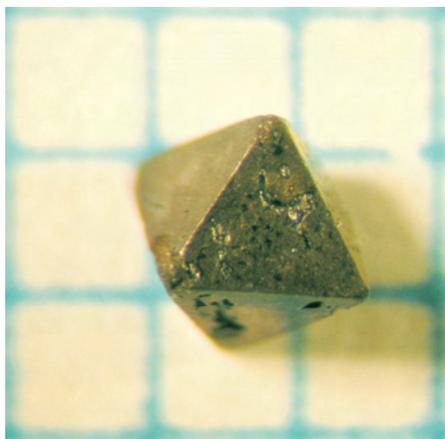
**Figure 18:** Single crystal of  $\alpha$ -pyrochlore  $\text{Na}_{1.6}\text{Os}_2\text{O}_{6.6}$  grown under high pressure.
