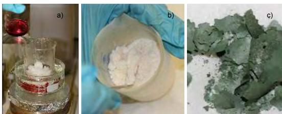
**Figure 5:** Synthesis of ZnO doped with transition metals by the nitrate route. The process is consisting in three steps: melting of nitrates (a), quenching to preserve the homogeneity of Mn distribution in a powder form (b), fast decomposition to produce the oxides (c).
