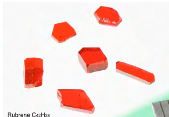
**Figure 17:** Typical single crystals of rubrene organic molecular crystal prepared by chemical vapor transport method.
