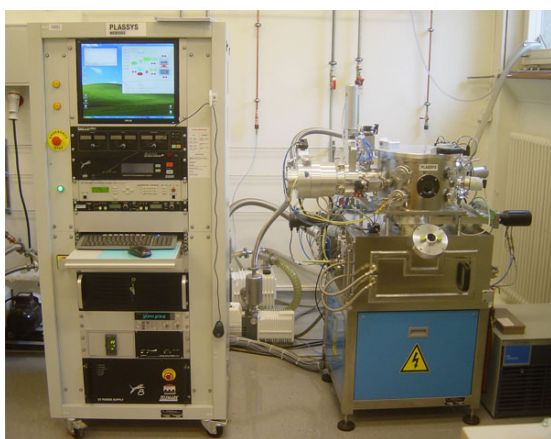
Figure 12: The new e-gun evaporator enabling the deposition of metallic films, as it is needed for the fabrication of nano-electronic devices.
