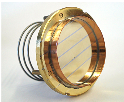
Figure 11: Brass plate with buried Fe-wires for magnetic separation and T_c measurements of small grains. The spring serves for vibrating the plate, thereby distributing grains over the buried wires.
