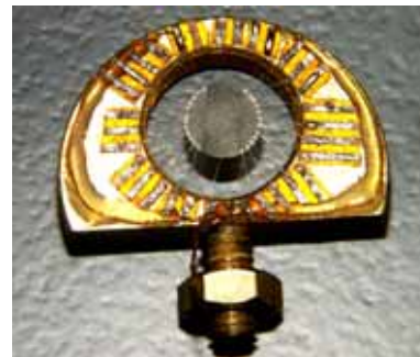
Fig.11. Combined heat-flow and AC calorimeter made of a sapphire disc equipped with a Au-Fe/Chromel thermopile.
