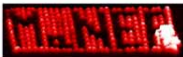
Fig.11. Array of 28x11 dots showing the word “MaNEP”. The density is about 6Gbit/cm 2 .
