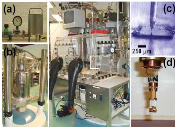
Fig. 7. The Calypso system with the glove box in front (center). (a) Detail of the annealing furnace. (b) Detail of the cryostat. (c) Tip-sample approach inside the glove box as seen with the optical system. (d) STM head.
